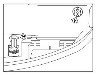
If you believe your headlamps need horizontal (H) (left/right) adjustment, follow the horizontal aiming procedure. If you believe your headlamps need only vertical (V) (up/down) adjustment, follow only the vertical aiming procedure.
